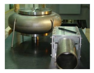
Figure D: Nb Half cells and end tubes assembled with the welding fixtures
