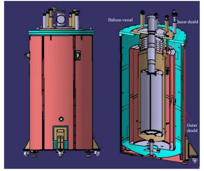
Model of test cryostat
