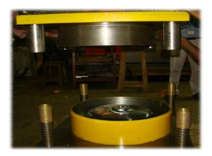
Figure C: Die-Punch for deep drawing trial
